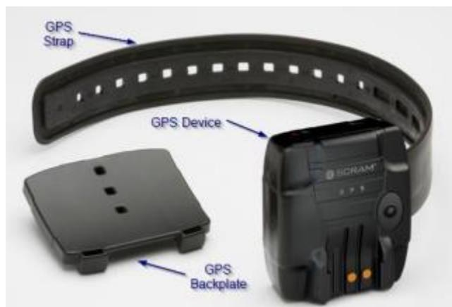
(236 grams), and is sealed and waterproof to two meters. The SCRAM GPS device has been tested and complies with military standards MIL-STD-810F Method 516.6 and IP-57 respectively for shock and water ingress and is FCC compliant (FCC ID P8M-GPS-600).
