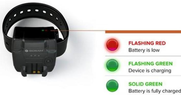
The internal battery is rechargeable and has visible LED lights on the device to show when the battery is low, charging, and fully charged.
