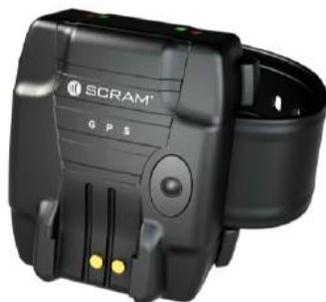
The SCRAM GPS® one-piece device is a slim, lightweight bracelet that attaches to the client's ankle and tracks movements 24/7. The device operates with a GPS background, tracking points as frequently as once per minute, and once every 15 seconds if the client enters an exclusion zone or if the officer manually activates Pursuit Mode. These location points can be transmitted via 4G LTE on the AT&T (GSM) or Verizon (CDMA) cellular networks per the communication frequency chosen by the County.
